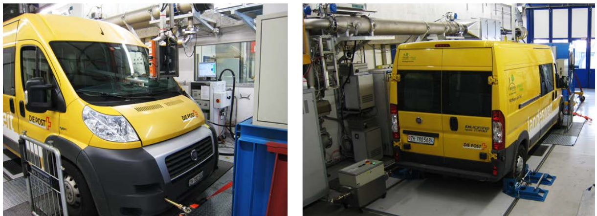
Fig. 5.10 Fiat Ducato from the Mobility Solution AG on the chassis dyno at Empa
