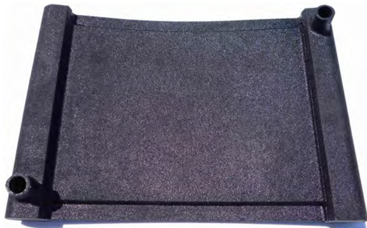
Figure 10.8: Functional model of the elastic heat exchanger printed in a 3D-printer.
