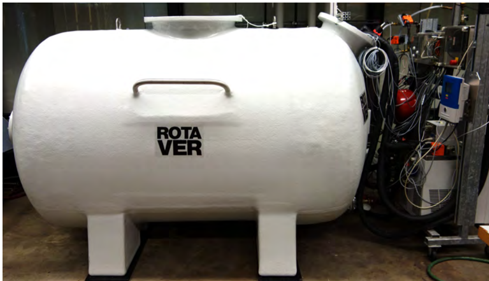
Figure 10.11: Test set-up for a cylindrical ice storage in laboratory.
