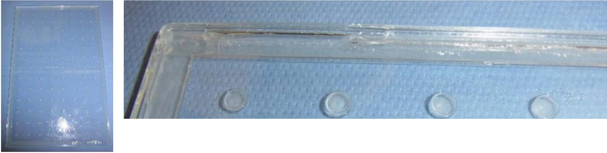
**Fig. 1.4.6: Sample 6 after test; cracks along boarder spacer (right)**
