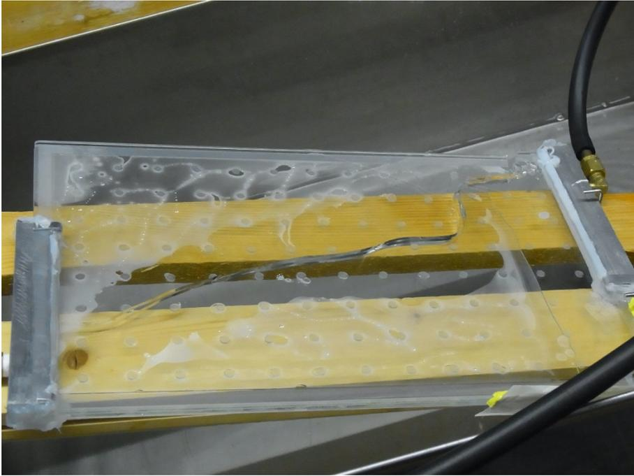
**Fig. 1.4.8: Borofloat sample after internal thermal shock.**
