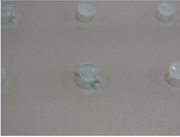
**Fig. 1.4.4: Damage of glass panes around centre spacer (typical for borofloat samples)**
