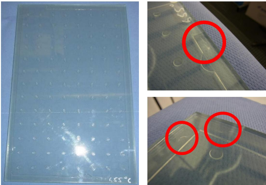
**Fig. 1.4.2: Sample 2 after test (left); cracks in spacer, (right)**
