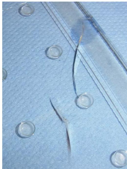
**Fig. 1.4.5: Sample 5 after test; large cracks in glass panes (right)**
