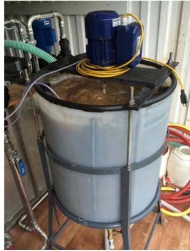
Figure 16. The 150L process tank used for aerobic granular biomass on-site cultivation.
