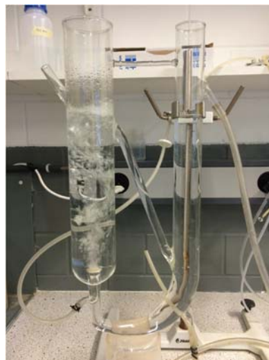
Figure 10. Glass column bioreactor of 1L used to favor the process of granular biomass cultivation.
