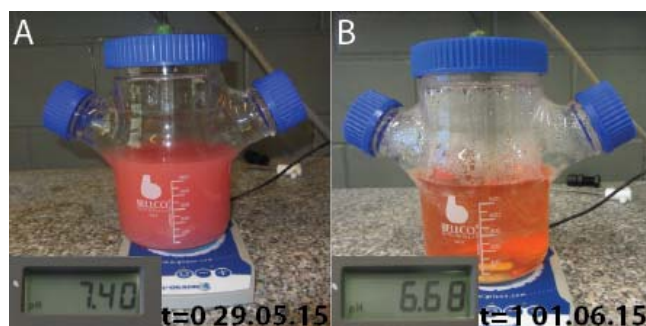
Figure 8. Glass bioreactor containing a culture of pre-enriched nitrifiers on GSN media at the starting point (A) and when the culture was stopped after 5 days (B). The image corresponds to the measurements of the pH probe.
