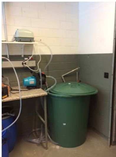
Figure 15. The 320L PVC tank used for aerobic granular biomass cultivation.
