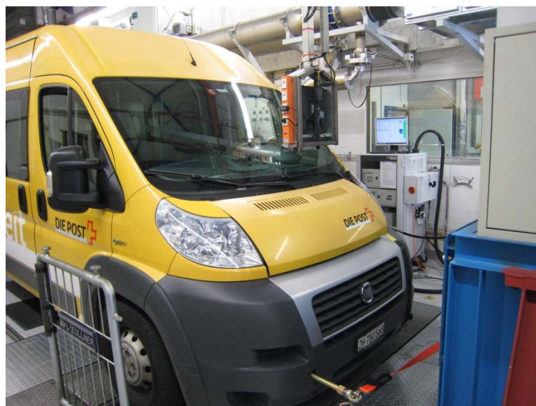
Fig. 3.2: Fiat Ducato from Mobility Solutions AG on the chassis dyno at Empa
