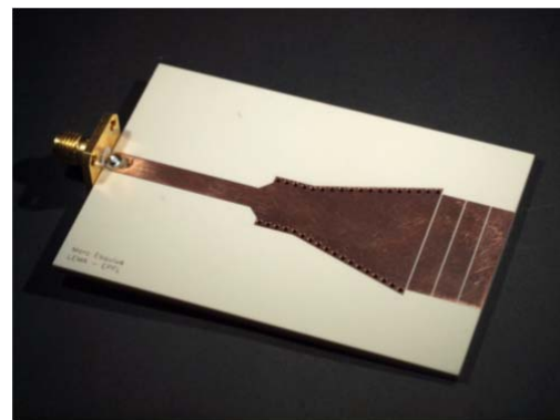
Figure 2 - Fully printed prototype of the SIW horn antenna
