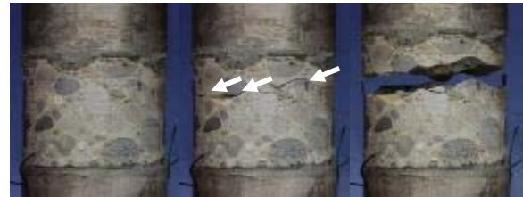
Result of a medium strain rate test on a cylinder of plain concrete.
