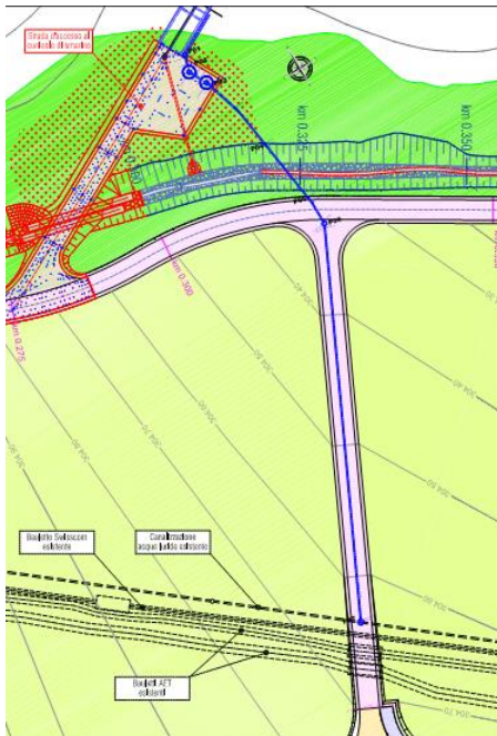
Fig. 5: Plant waste water pre-treatment installations and connection to the communal sewage system at the Pollegio portal. Left: Situation of the installations shown on map (indicated in blue). Right: Picture of the pre-treatment plant.
