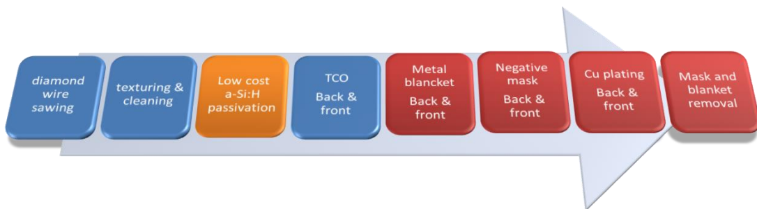
Figure 1.14: process flow of Si-HJT Gen 3.3 plated cells
