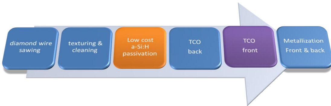
Figure 1.9: process flow of Si-HJT Gen 2 cells
