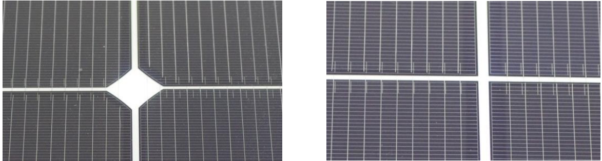
Figure 2.15: on left, picture of a regular SWCT module based on PSQ cells, the white diamond shape between cells produces no power. On right, rectangular shape cells leave minimal area between the cells, high cell density in module.
