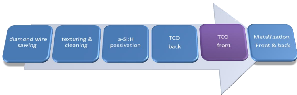
Figure 1.5: process flow of Si-HJT 2.0 Gen 3 cells
