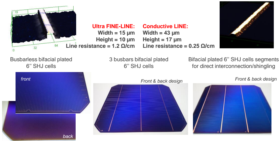
Figure 2.10: Pictures of full wafer 6" silicon heterojunction cells with the different plated metallization grid patterns defined, respectively for busbarless bifacial cells, 3 busbars bifacial cells and bifacial cells with specific design for cell segmentation followed by direct interconnection ("shingling").
