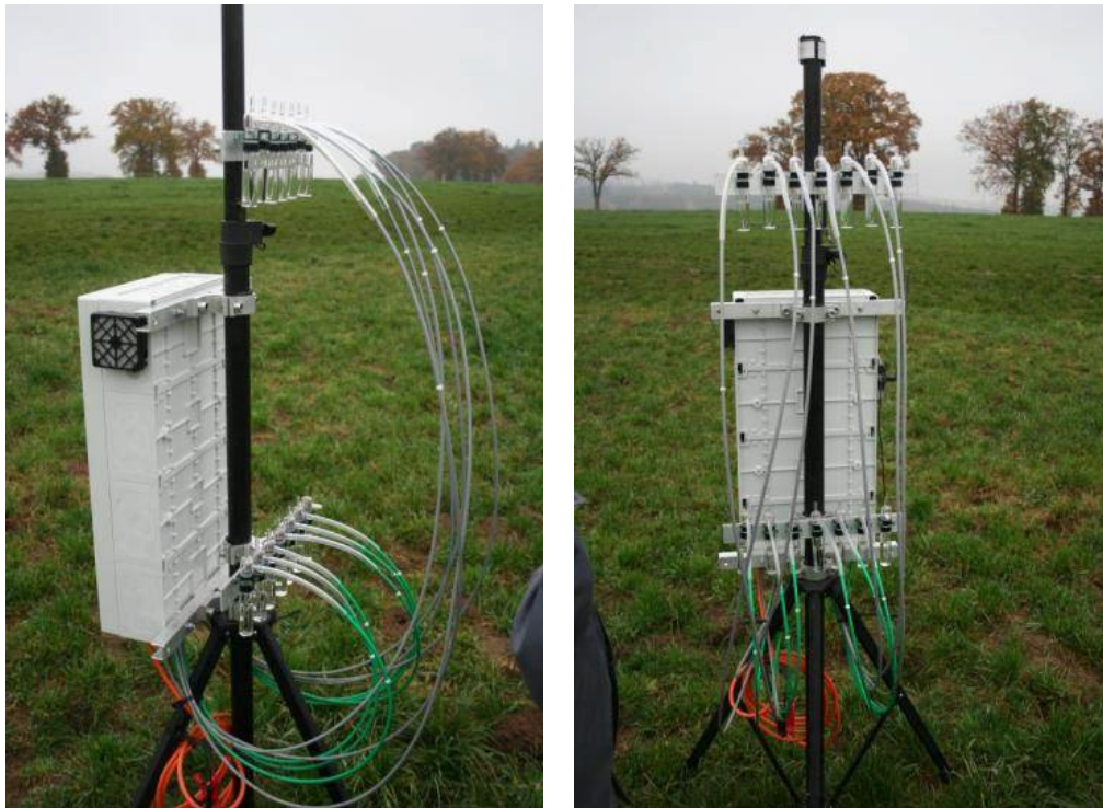
Abbildung 4: NH 3 -Messsysteme: Low-Cost Impinger Sampling Device (LOCI).
