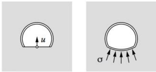
In tunnelling, the swelling causes a long-term heave of the tunnel floor, which may impair the serviceability of the structure (a). On the other hand, when attempting to prevent floor heave by means of an invert arch, so-called swelling pressure develops, which may damage the tunnel lining (b).
