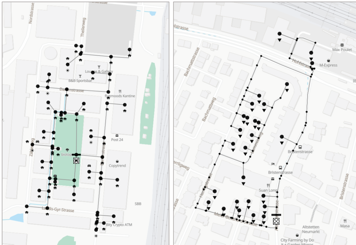
Figure 12: Synthetic grids for two sample areas in Zug (left) and Zurich Altstetten.
