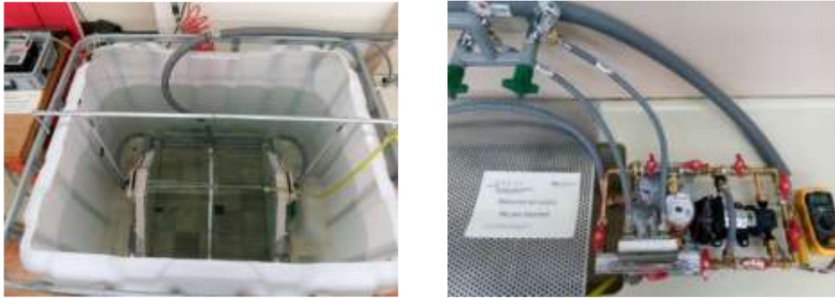
Figures. 21 & 22: ULISSE Mock-up in the IBC test tank connected to the hydrothermal supply unite (HSU)
