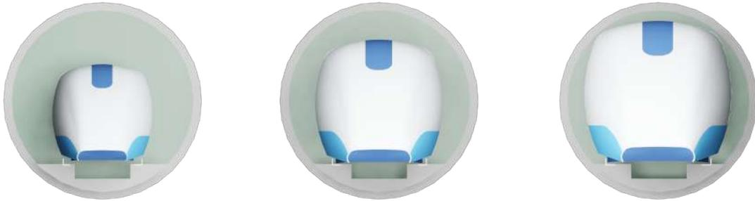
Figure 16: Left to right: Blockage ratios of 0.36, 0.6 and 0.83: Ratio of the inner area of the tube that pod and sleeper occupy together.
