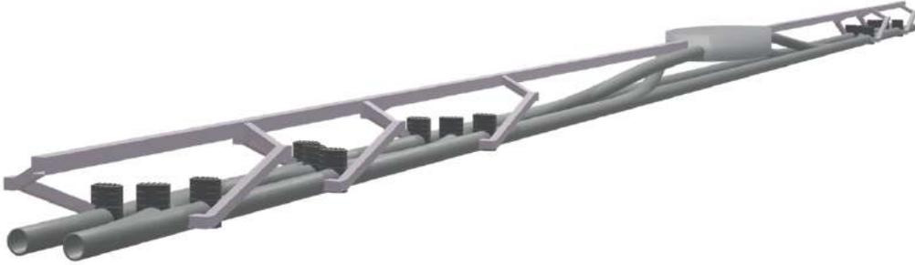
Figure 19: Underground system for a hyperloop with bypass system, valves, on-/off-ramps and safety tunnel above the main line
