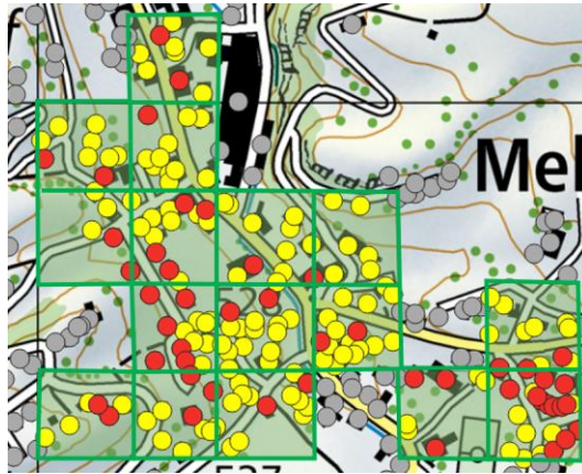
Figure 3: Example of a raster field that is considered as the territory of the district. The red points indicate the buildings connected to the network, the yellow points the remaining buildings within the raster field and the grey points the remaining buildings that were not considered as they are not enclosed by the field.
