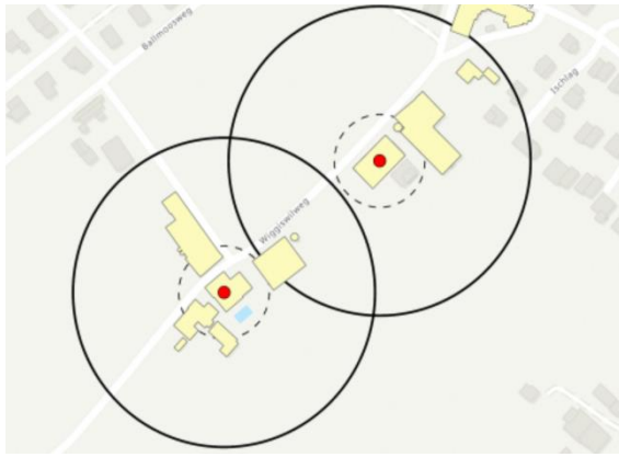
Figure 1: Identification and assignation of roofs of agricultural buildings in relation to the closest farm to estimate the local PV potential.
