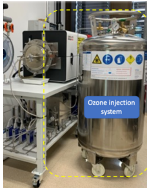
Figure 6. Ozone reservoir for a quick injection of ozone into the CVD furnace.
