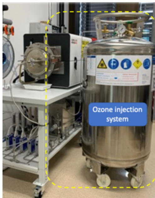
Figure 12. Ozone reservoir for a quick injection of ozone into the CVD furnace.
