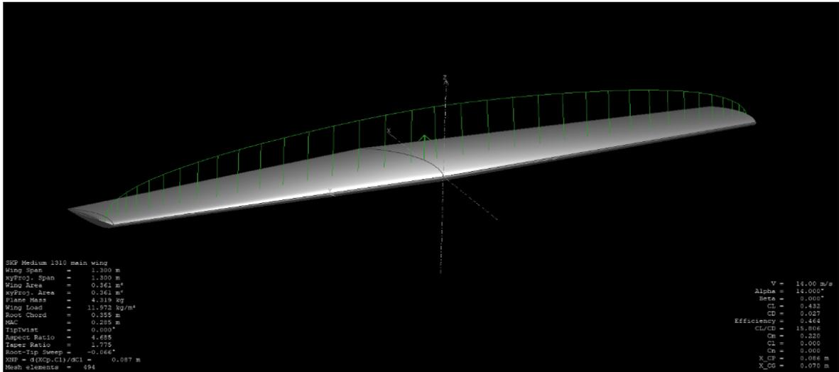
Figure 24: Load Distribution in the Main Wing
