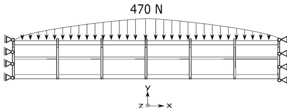
Figure 37 SP 180- 01 Main Wing boundary and loading conditions
