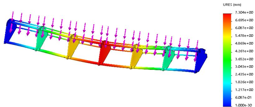
Figure 39 Maximum Displacement for loading conditions
