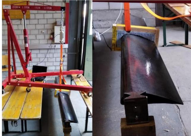
Figure 46: Static test on the main wing of SP180-01 on the new test bench
