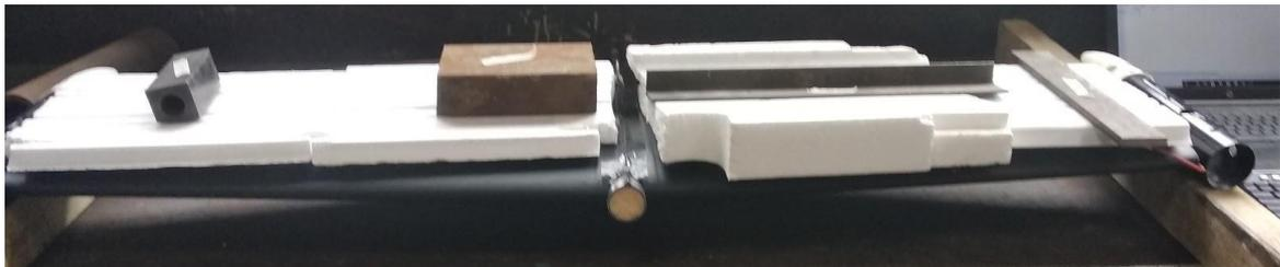
Figure 44: Polystyrene slabs placed on main wings of 130-02
