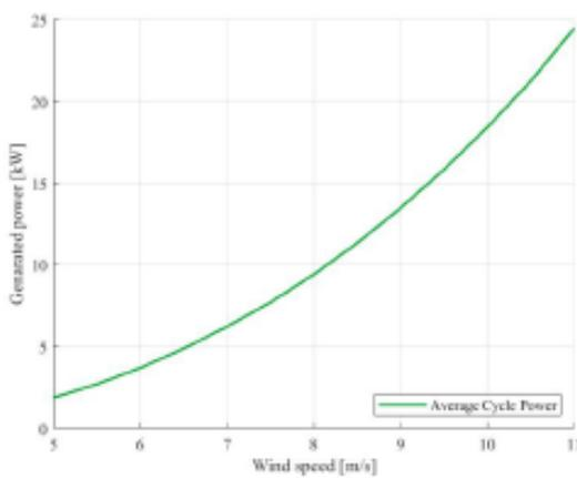
Figure 10: Computed power curve of a 3.2m UAV
