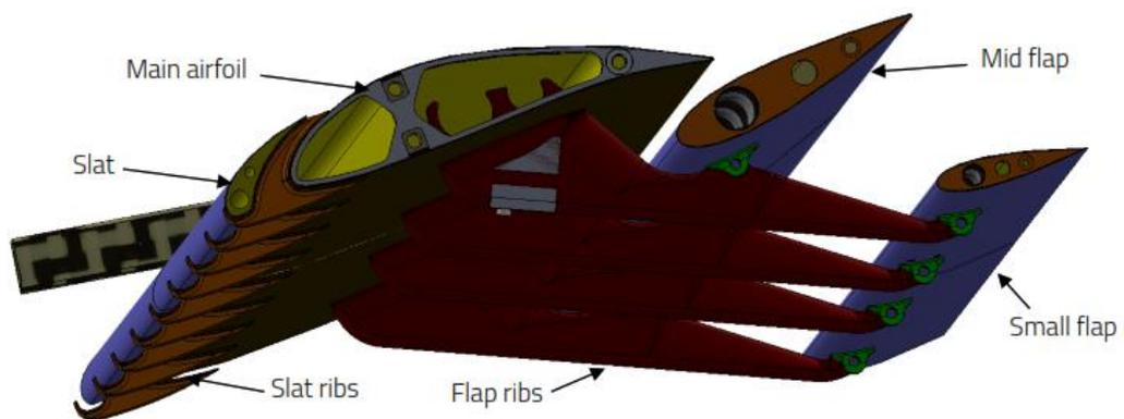
Figure 40 Modified SP180 main wing design
