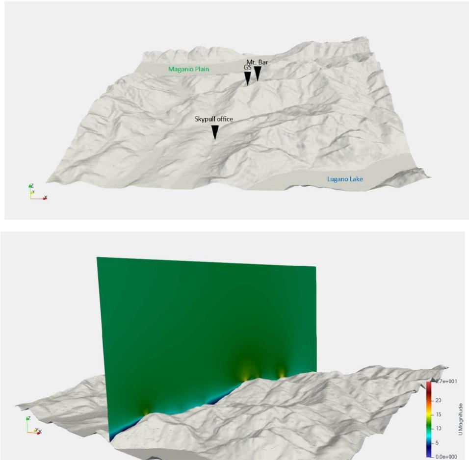
Figure 8: Discretized region in grey and a slice in north-south direction of the flow field in m/s.
