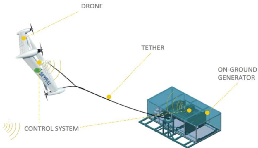
Figure 1: Overall Schematic diagram of Skypull Technology
