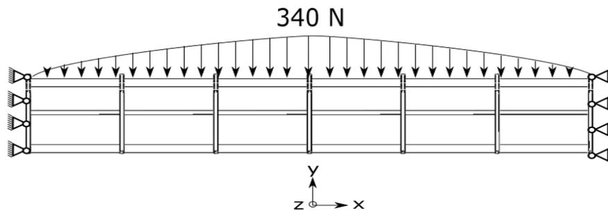
Figure 29: static load simulation
