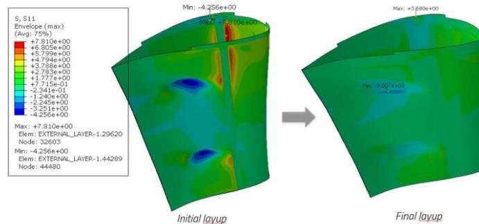
Figure 42 Study on reduction of stresses on external fibres layers on the SP180 main wing due a new layup
