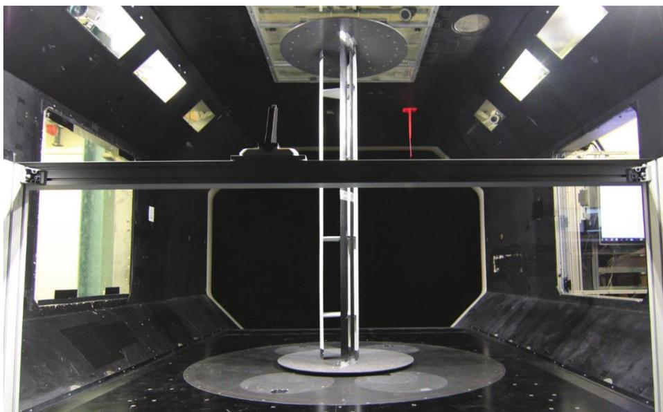
Figure 47: Aerodynamic test of the Skypull SP180 airfoil within the ETH wind tunnel facility
