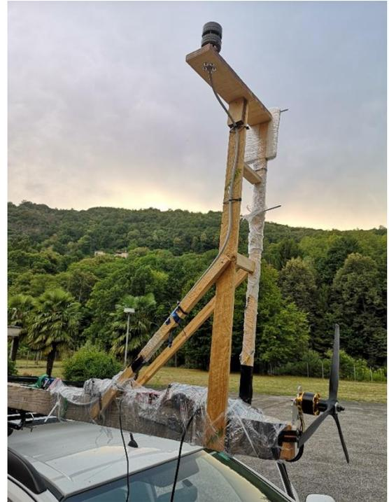
Figure 18: The system used on car to test regeneration performances
