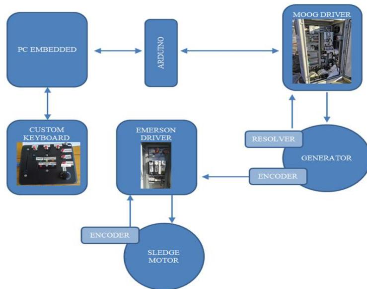
Figure 62: Ground Generation System Scheme
