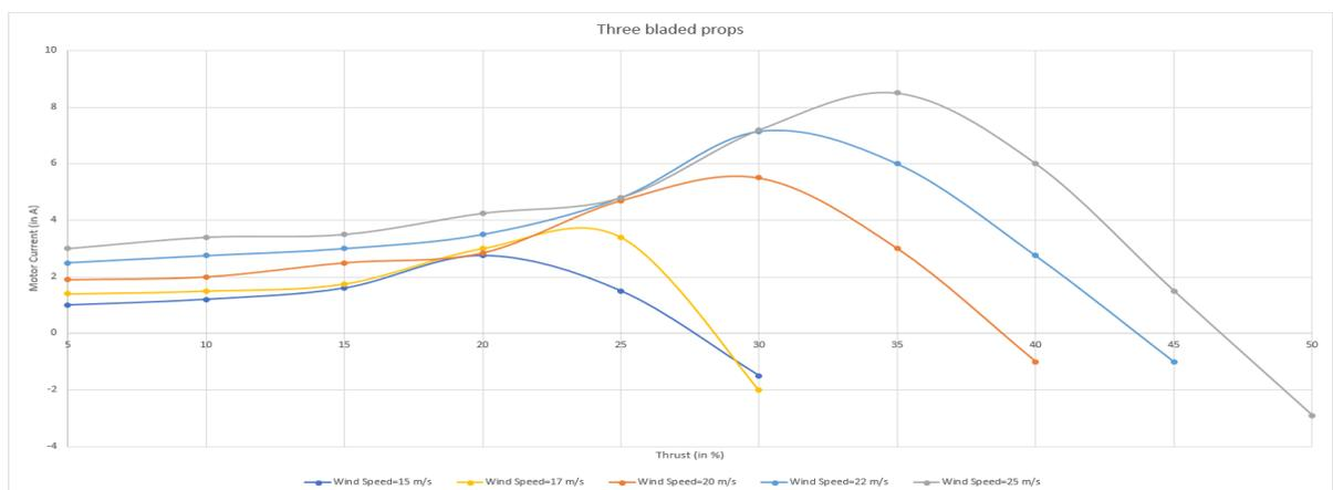
Figure 17: Regeneration curves at multiple air speeds
