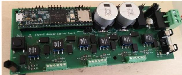
Figure 71: Teensy 3.6 Control Board
