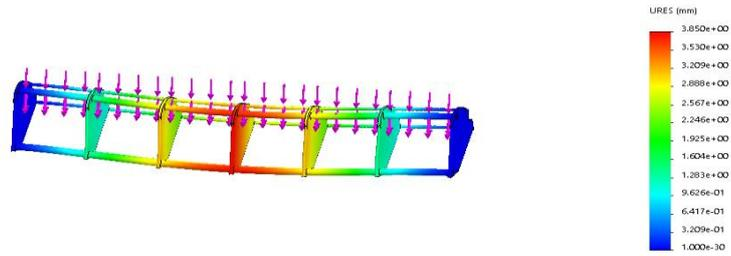
Figure 33: Maximum Displacement for loading condition
