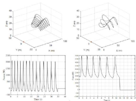
Figure 10: example of computed pumping cycle
