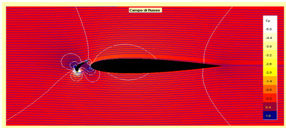
Figure 25: CFD analysis with infinite airfoil for four propellers
