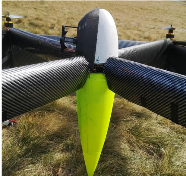
Figure 53: UAV ultrasonic wind sensor implemented
