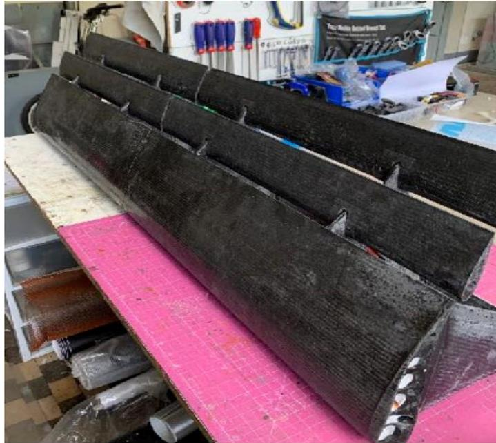
Figure 56: SP130-03 Main wing construction
