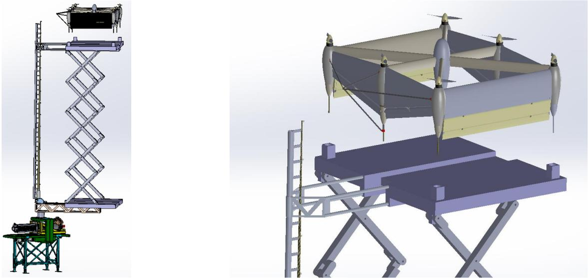
Figure 65: Study of a Ground Station with take-off /landing platform
