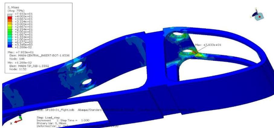
Figure 41 FEM analysis on Mises stress on central insert of lower main wing
