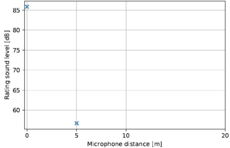
Figure 13: TO&L UAV recorded sound levels
