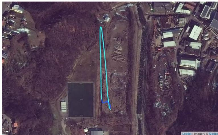
Figure 76: Autonomous return to home (straight line) flight test of a UAV
