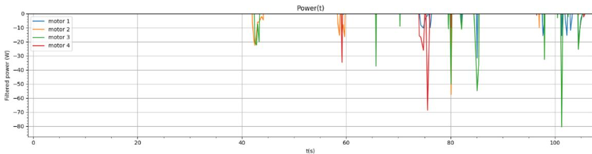
Figure 16: VESC power consumption plot (negative values represent power generation)
