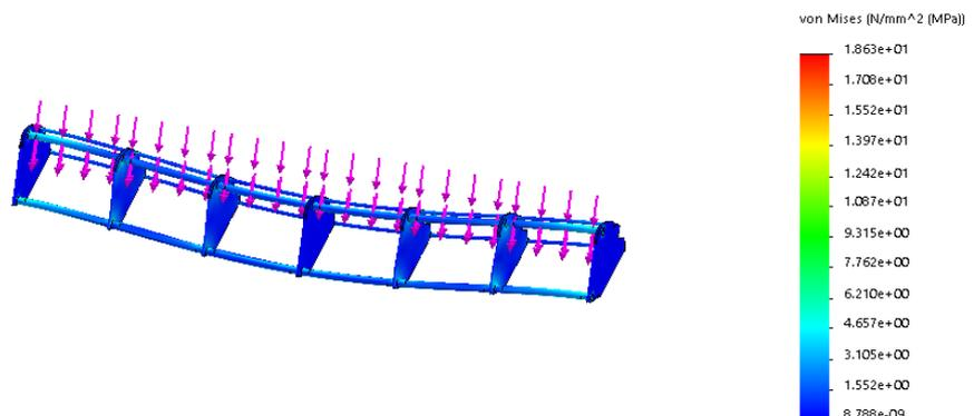
Figure 38: SP 180- 01 Main Wing Von Mises Stress distribution for loading conditions
