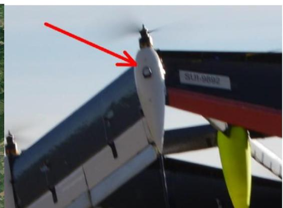
Figure 5: Flashing strobo lights mounted on Skypull's UAV
