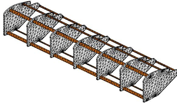
Figure 30: Main wing meshed component
