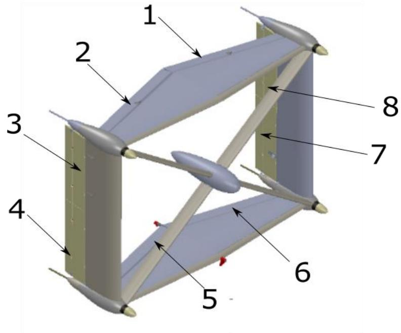
Figure 26: Flight Control Surfaces of SP130-02
