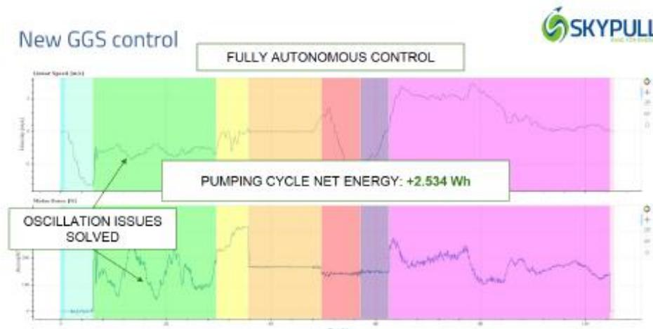
Figure 68: Result obtained by using the new GS control strategy
