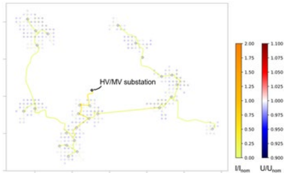
Figure 3.2.1: Distribution grids routing: Medium voltage grid under nominal operation and reports per-unit voltage of buses and current conductors.
