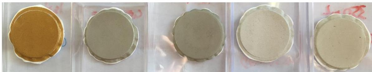
Figure 10: Filtered samples of suspended particle loads collected after producing for 0.04, 0.24, 0.44, 1.01, and 3.87 well volumes (from left to right). The colour difference relates to a variation of the
