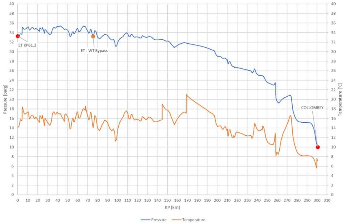
Figure 8.2.5: Gaseous Phase Transport to Collombey. Trunklines Pressure and Temperature Profiles.
