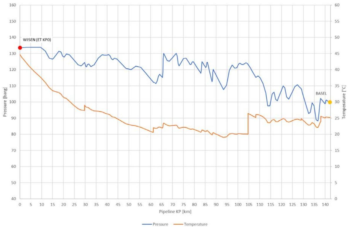
Figure 9.2.2: Dense Phase Transport. East Trunkline Pressure and Temperature Profiles.
