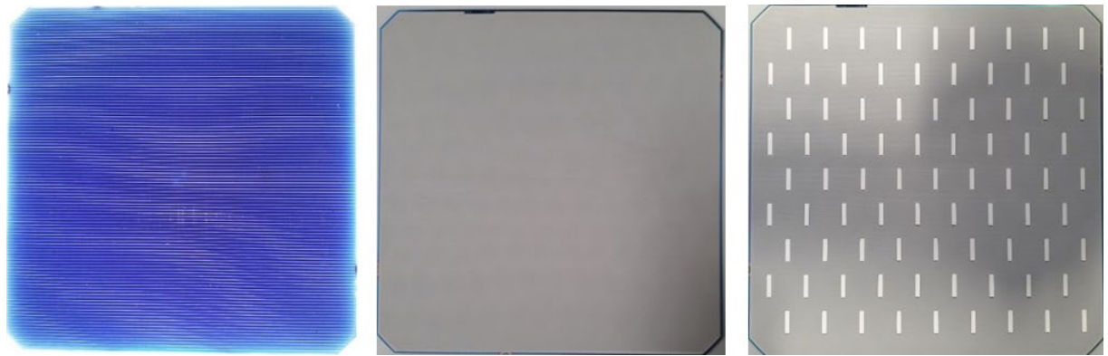
Figure 17: Monofacial PERC cells. Left: front side; middle: full aluminium rear side; right: rear side with Ag pads. (Run 3106)
