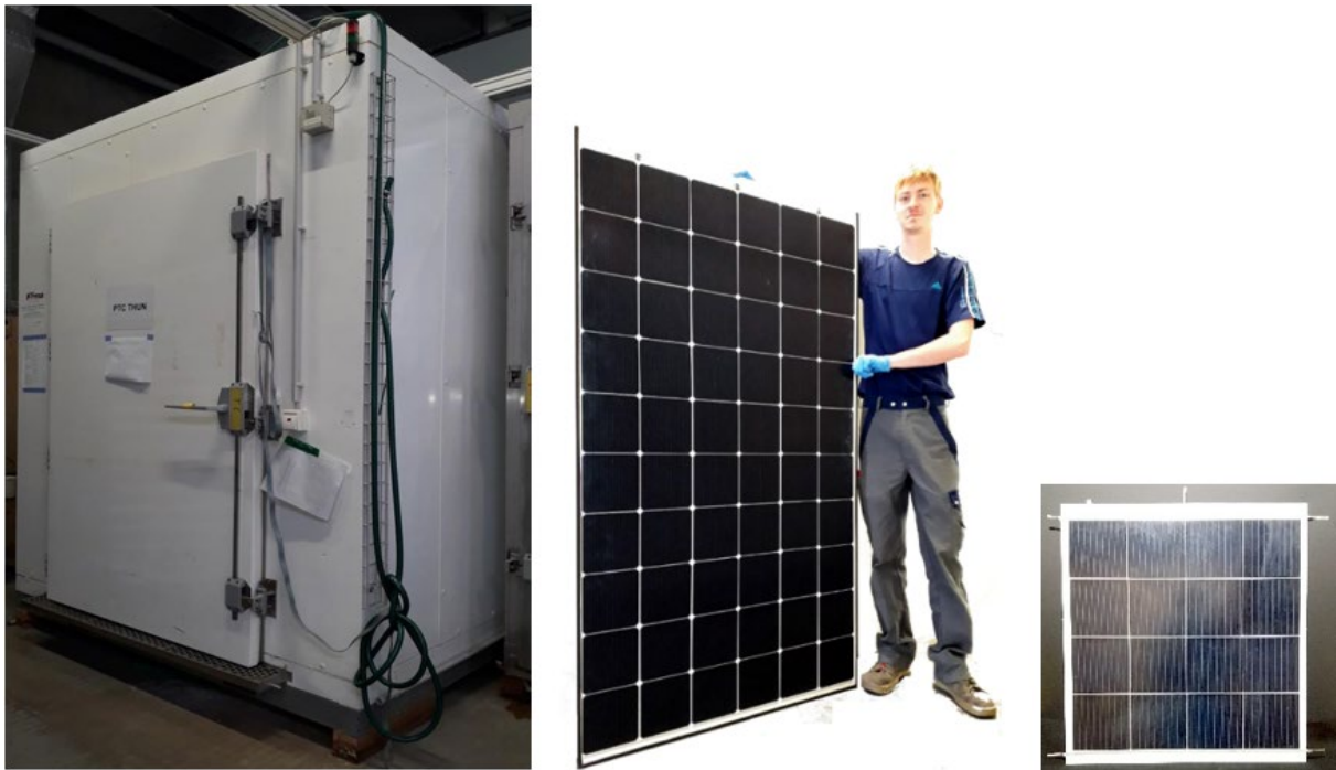
Figure 11: Left: Climatic chamber (PTC, DH). Middle/right: Examples of 60-cells, and 16-cells modules.
