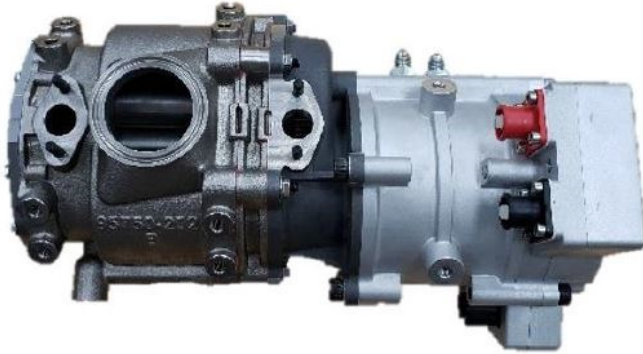
Figure 15: Dedicated EGR pump prototype with integrated 48V e-motor from Eaton
