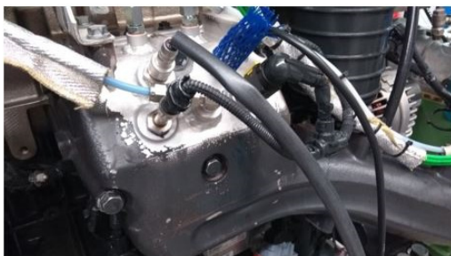
Figure 18: Lambda sensor LSU5.1 used in the Intake Manifold
