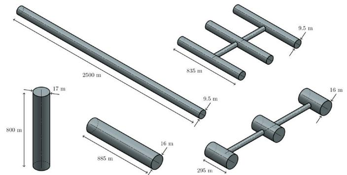
A commercial compressed air storage plant with a capacity of 500 MWh would require a rock cavern with a volume of 177,000 m<sup>3</sup>, which corresponds to a sphere with a diameter of 70 m. Apart from a sphere, other shapes are also conceivable, as shown in the diagram. Which shape is most suitable is being investigated in a SFOE project that is currently still ongoing. Illustration: Philipp Roos / Andreas Haselbacher
