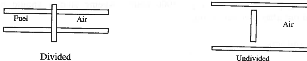
Simplified divided and undivided cell configurations
