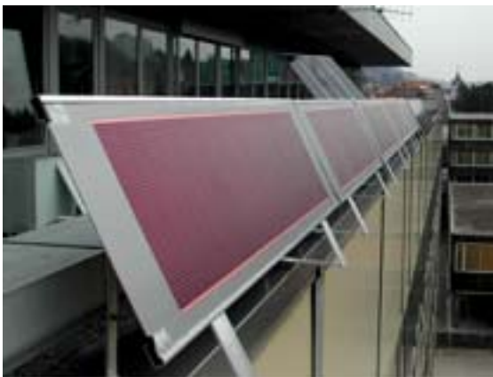
Figure 4: Initial solar module prototypes based on Alucobond ® and VHF Technologies' amorphous silicon solar cell being tested at the University of Applied Sciences in Le Locle (photo: EIAJ)
