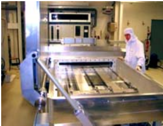
Figure 1: Industrial KAI plasma deposition plant (Photo: Unaxis)
