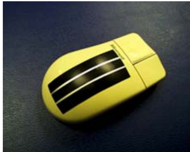
Figure 9: Application of the polymer solar battery (Photo: Varta)
