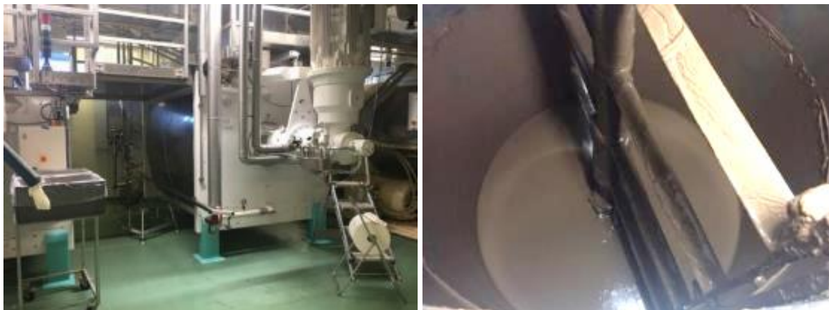
Figure 17: Large conching machine in production. Agitator to keep the chocolate mass warm at 45 °C.
