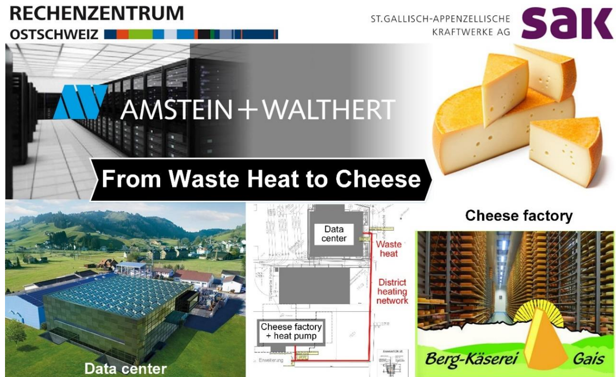
Figure 12: Waste heat from the server cooling of the data center is fed into a district heating network at around 20 °C. The mountain cheese factory utilizes this waste heat as heat source in a HTHP to generate process heat for the cheese production [16].
