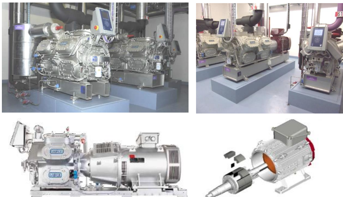
Figure 46: Ammonia compressors from Johnson Controls of brand Sabroe (HPC version 106S, 40 bar) with permanent magnet motors and electronic variable speed inverters [40,42].
