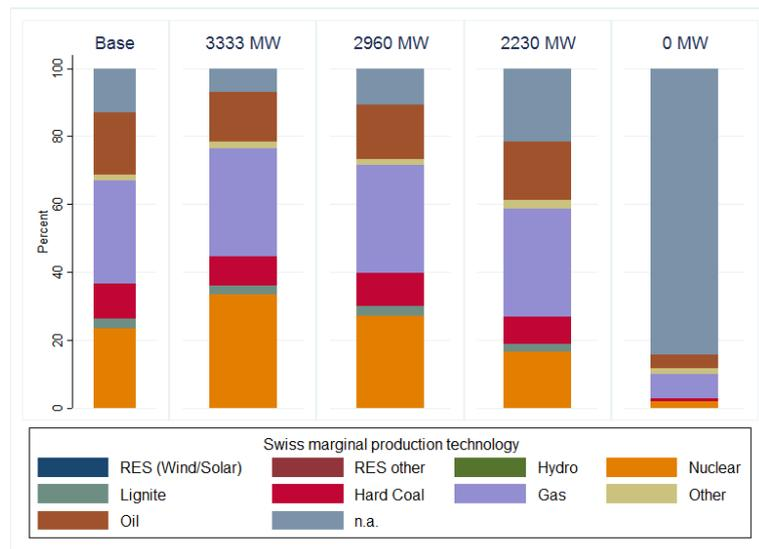
**Figure 15: Share of production technology: nuclear phase-out (scenario 2a)**
