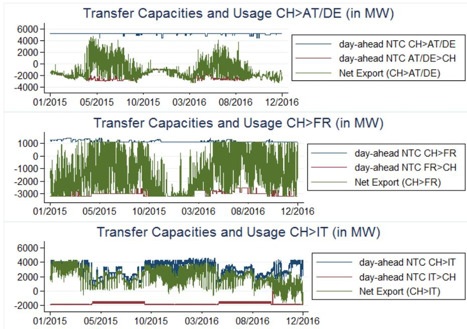
**Figure A-1: Transfer capacities and usage by border**
