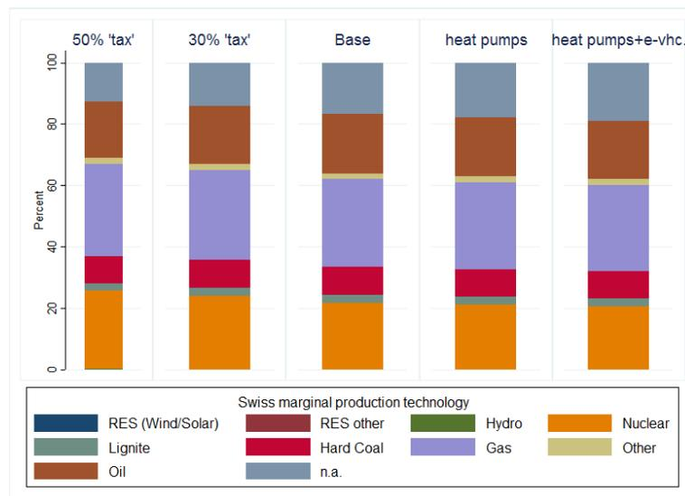
**Figure 23: Share of production technology: load (scenario 2c)**
