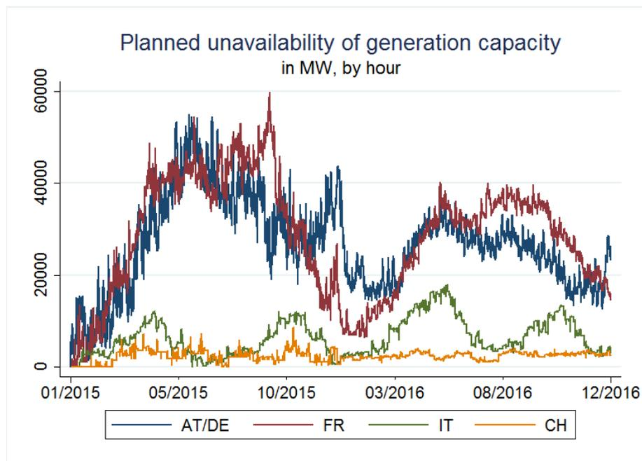
Figure A-4: Unavailable generation capacity
