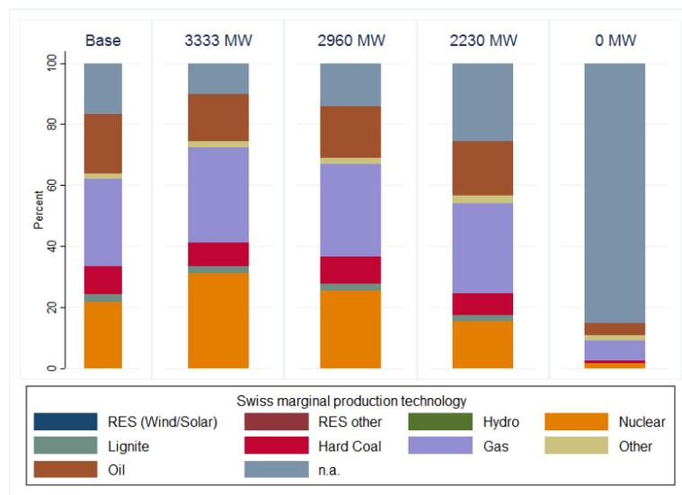
**Figure 27: Share of production technology: nuclear phase-out (scenario 2c)**
