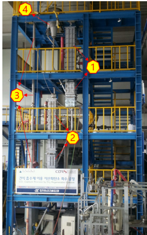
Figure 3. Illustration of the 100 kg scale fluidised bed continuous unit; 1) the sorption reactor, 2) the desorption reactor, 3) the solid transport system (riser), 4) the main cyclone.
