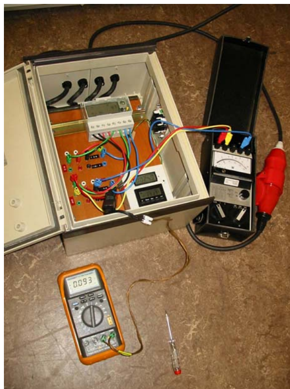
Fig. 3.2 Equipment for measuring standby consumption (EMU 32 3-phase, adaptable inputs/outputs, moving-coil wattmeter, sensor, multiple measurement device)
