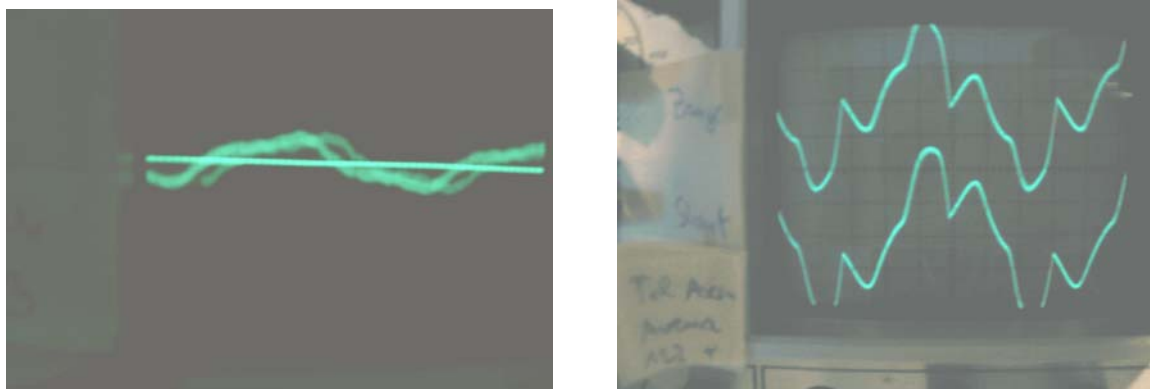
Fig. 3.1 Oscillograph showing current flows: a) air-flow clothes dryer, approx. 0.4 W (left) b) mobile phone, 4.5 W (right – upper curve = fork sensor, lower curve = shunt)
