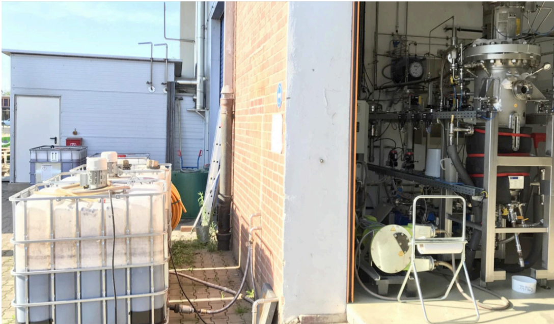
The German company microbE-nergy carried out laboratory tests with sewage sludge from the Reinach WWTP. The tests showed that this substrate is suitable for biological methanation. Photo: microbEnergy.
