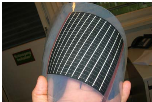
Figure 4: Flexible monolithic demonstrator modules with grid interconnected cells (photo: FLISOM).
