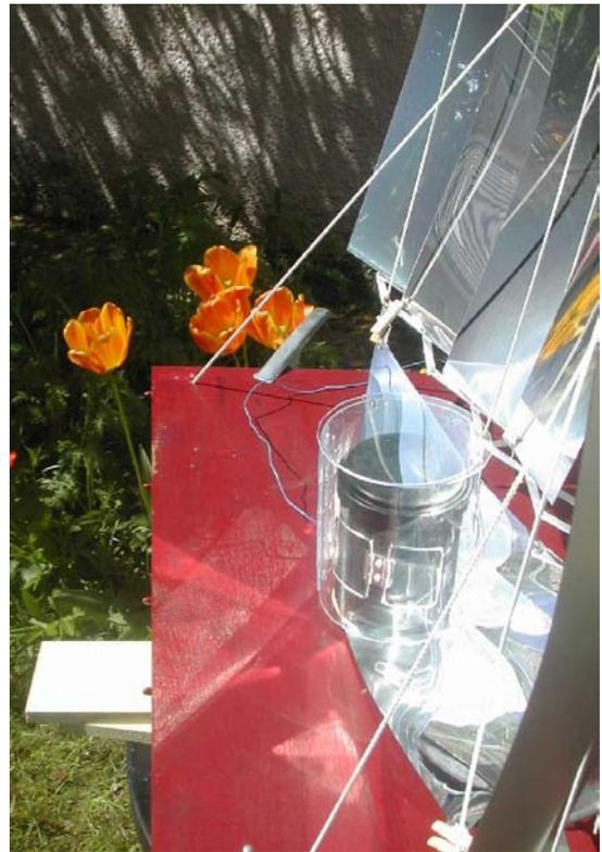
*Figure 6. A polycarbonate windshield protects the cooking vessel.*
